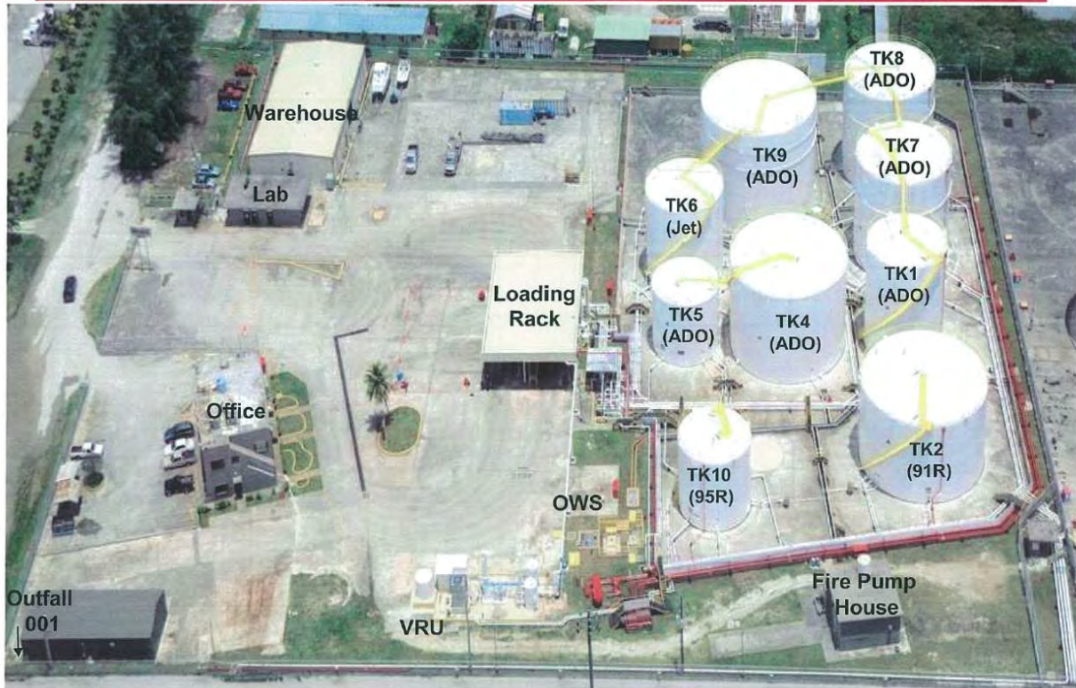
Figure 3. Site map of Mobil Saipan Terminal. Shows location of Outfall 001 and oil-water separator (OWS).
